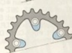
Chain protection guards for easy re-mounting of thrown chains (inner)
